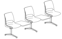
Three Seats and Two Inline Tables W108" H33" Seat: W19.25" D18.75" H17"
